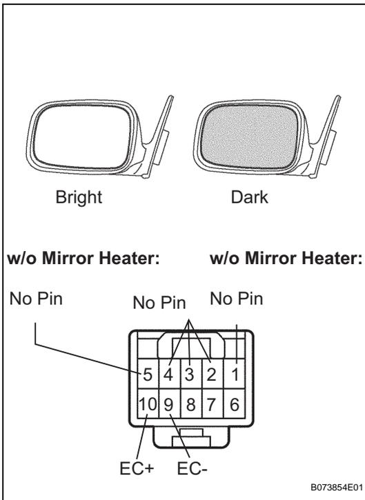
**3. INSPECT OUTER REAR VIEW MIRROR ASSEMBLY LH (w/ EC Mirror)**
