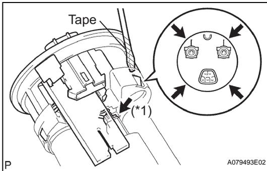
**12. REMOVE FUEL SUCTION PLATE SUB-ASSEMBLY**
