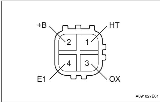
**4. INSPECT OXYGEN SENSOR (BANK 1 SENSOR 2)**
