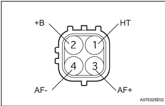
**3. INSPECT AIR FUEL RATIO SENSOR (BANK 1 SENSOR 2)**
