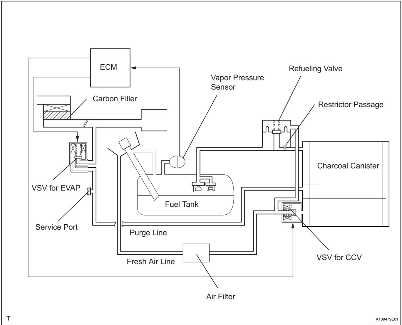
The emission control system is determined by the ECM based on signals from various sensors.
