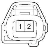
C4 Crankshaft Position Sensor
