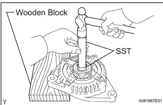
(b) Using SST, tap out the bearing.
