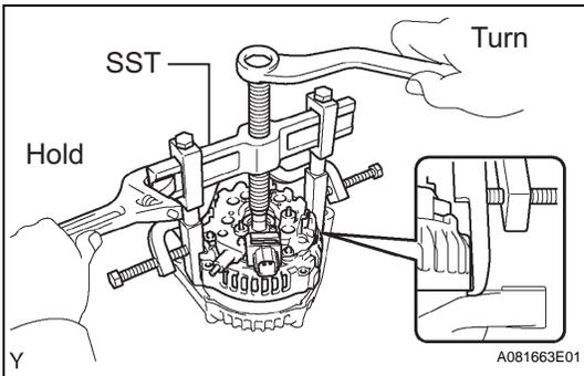
(b) Using SST, remove the generator rectifier end frame.
