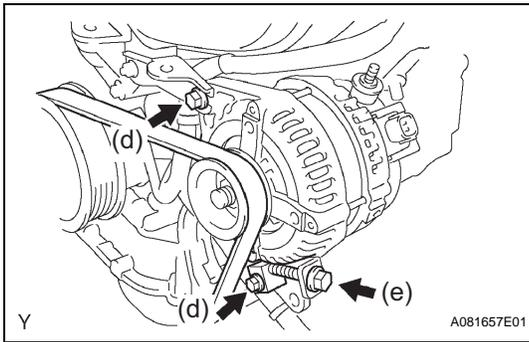
(b) Adjust the V belt tension by tightening the bolt.
