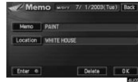
Touch the corresponding date. Touch the corresponding memo switch, and then touch the “Delete” switch on the screen. A message appears on the display. To delete, touch the “Yes” switch. To cancel the deletion, touch the “No” switch.
