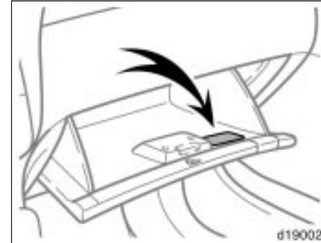
**The air conditioning filter information label is placed in the glove box as shown and indicates that a filter has been installed.**
