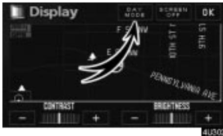
Depending on the position of the headlight switch, the screen changes to either day mode or night mode.
