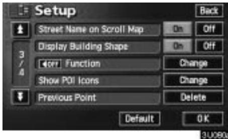
3. Touch the “On” switch of “Street Name on Scroll Map” and touch the “OK” switch.
