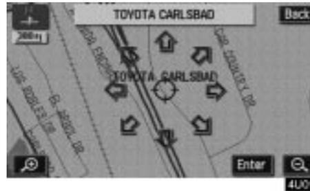
Set the cursor
