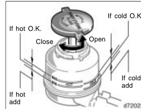
Check the fluid level through the reservoir. If necessary, add automatic transmission fluid DEXRON<sup>®</sup> III or III.
