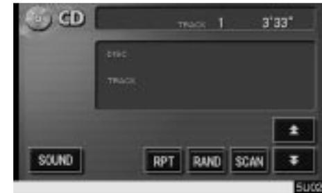
The switches for radio and compact disc player operation are displayed on the function switch display screen when the audio control mode is selected. Touch them lightly and directly on the screen.
