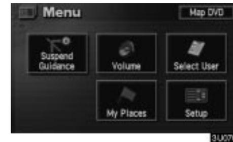
2. Touch the “Setup” switch. Then touch
