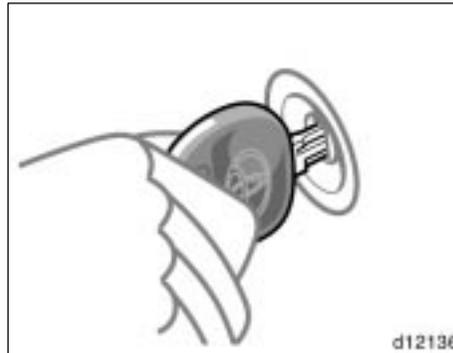
The engine immobilizer system is a theft deterrent system. When you insert the key in the ignition switch, the transponder chip in the key's head transmits an electronic code to the vehicle. The engine will start only when the electronic code in the chip corresponds to the registered ID code for the vehicle.
