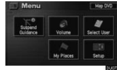
2. Touch the “Setup” switch. Then touch
