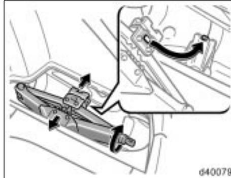
To store the jack, align the hole of the jack head with the vehicle hook. Turn the jack joint clockwise until the jack base fits securely with the vehicle body.
