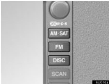
Push “AM-SAT”, “FM” or “DISC” button to turn on the desired mode. The selected mode turns on immediately.
