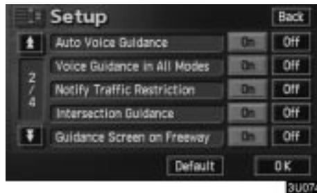
3. Touch the “On” switch of “Intersection Guidance” and touch the “OK” switch.
