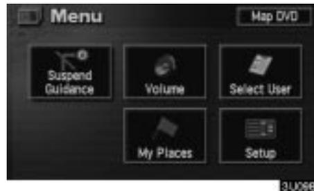
2. Touch the “Setup” switch. Then touch
