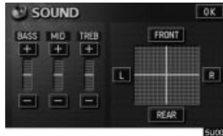
**Touching the “SOUND” switch displayed on the screen at the audio control mode will display the sound control mode. Adjust the tone and balance as follows.**
