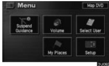
2. Touch the “Setup” switch. Then touch
