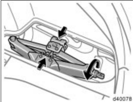
To remove the jack, turn the jack joint counterclockwise by hand until the jack becomes free.
