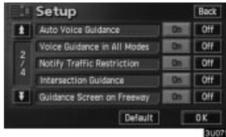
3. Touch the “On” switch of “Notify Traffic Restriction” and touch the “OK” switch.
