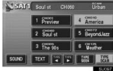
**To scan the currently selected channel category:** Touch the “TYPE SCAN” switch or push the “SCAN” button briefly. “SCAN” appears on the display. The radio will find the next channel in the same channel category, stay there for a few seconds, and then scan again. To select a channel, touch the “TYPE SCAN” switch or push the “SCAN” button a second time.
