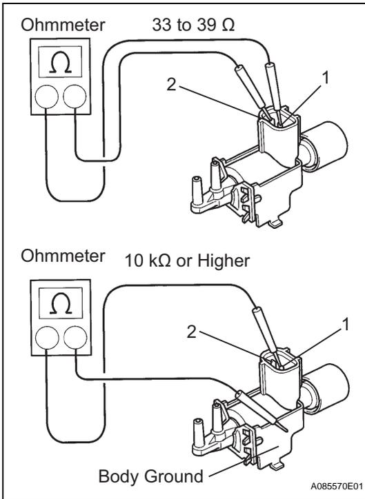
**4. INSPECT VACUUM SWITCHING VALVE FOR IAC VALVE ASSEMBLY NO.2**
